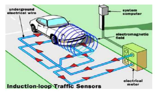
Figure 2.1. How an inductive loop detector works.
