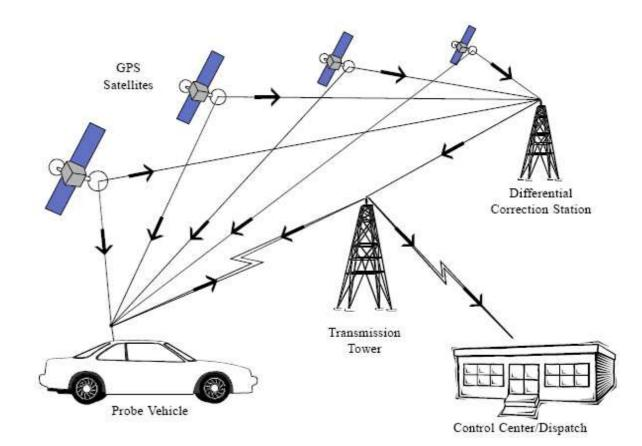
Fig 2.3. Probe vehicle system
