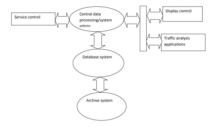
Figure 4.1. Components of the central operations and analysis system
