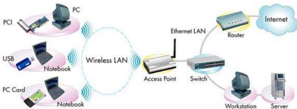
Figure 3: Wireless LANs with infrastructure mode. Source: EUSSO
