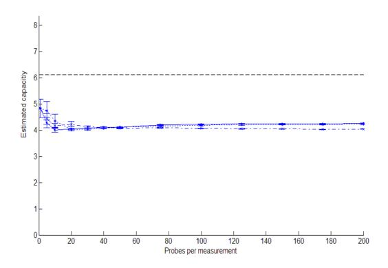
Figure 5.7illustrates the' single wireless' capacities of the network path using three related methods for filtering the measured RTTs. The probe method nearing path capacities of 4.2 Mbps. These are estimations are dependent on the amount cross-traffic in the link.
