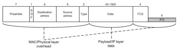
Figure 4.1 : Ethernet overhead
