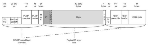
Figure 4.2 : An illustration of Overhead of 802.11b
