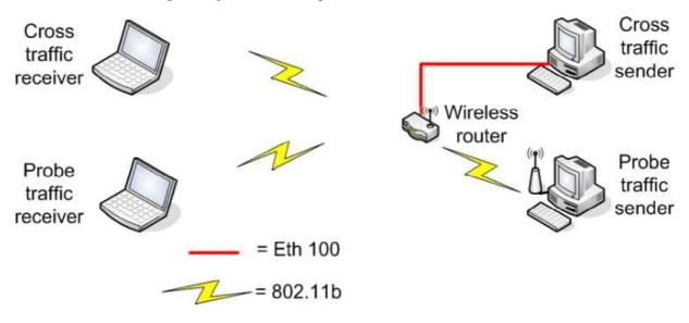
Figure 5.4: Simulated network with 802.11
