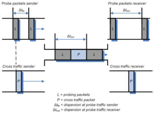
Figure 3.1: The "probe gap model" illustration.
