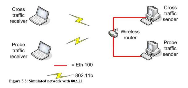
Since the wireless link is shared by the 'probe-traffic-receiver' and the 'cross-traffic-receiver', the capacity of the media is shared as well.
