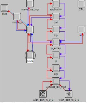
Figure 5.2:a node implementation in OPNET modeler
