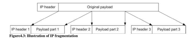
If any transitional nodes in the data path do not have the full support for fragmentation of IP, then packets bigger in size that the MTU-sized packets will not be forwarded but will otherwise be dropped and possibly error message response sent to the source node.
