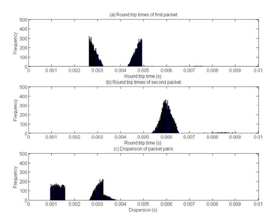
Figure 5.5: RTTs and dispersion of packet pairs in a "single wireless"
