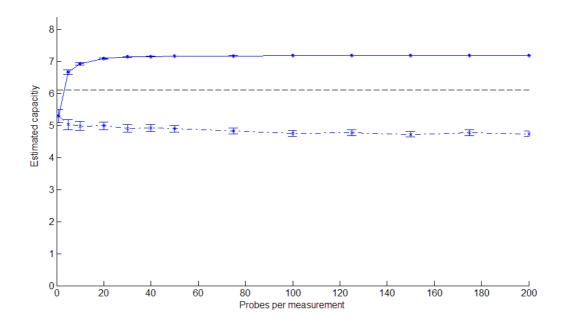
Figure 5.8: Single wireless path capacities estimation
