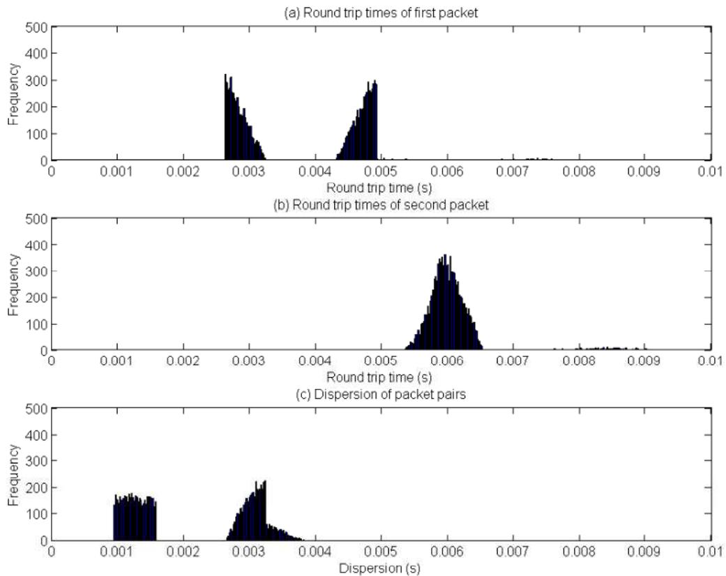
**Figure 5.5: RTTs and dispersion of packet pairs in a “single wireless”**
