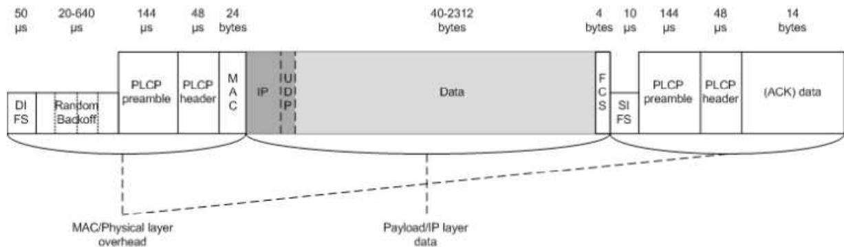
**Figure 4.2 : An illustration of Overhead of 802.11b**
