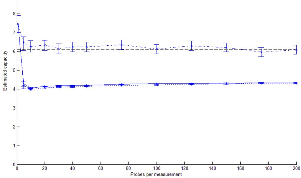
**Figure 5.6 : Estimated path capacities vs ppm for the “single wireless” scenario**
