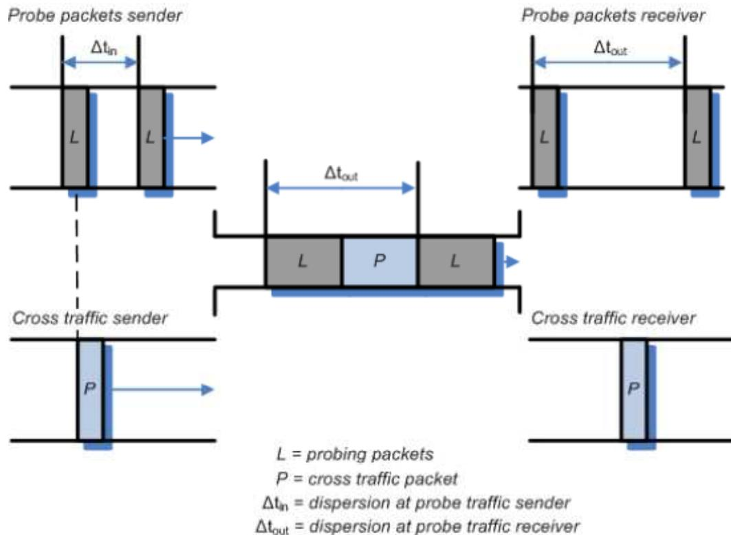
**Figure3.1: The “probe gap model” illustration.**
